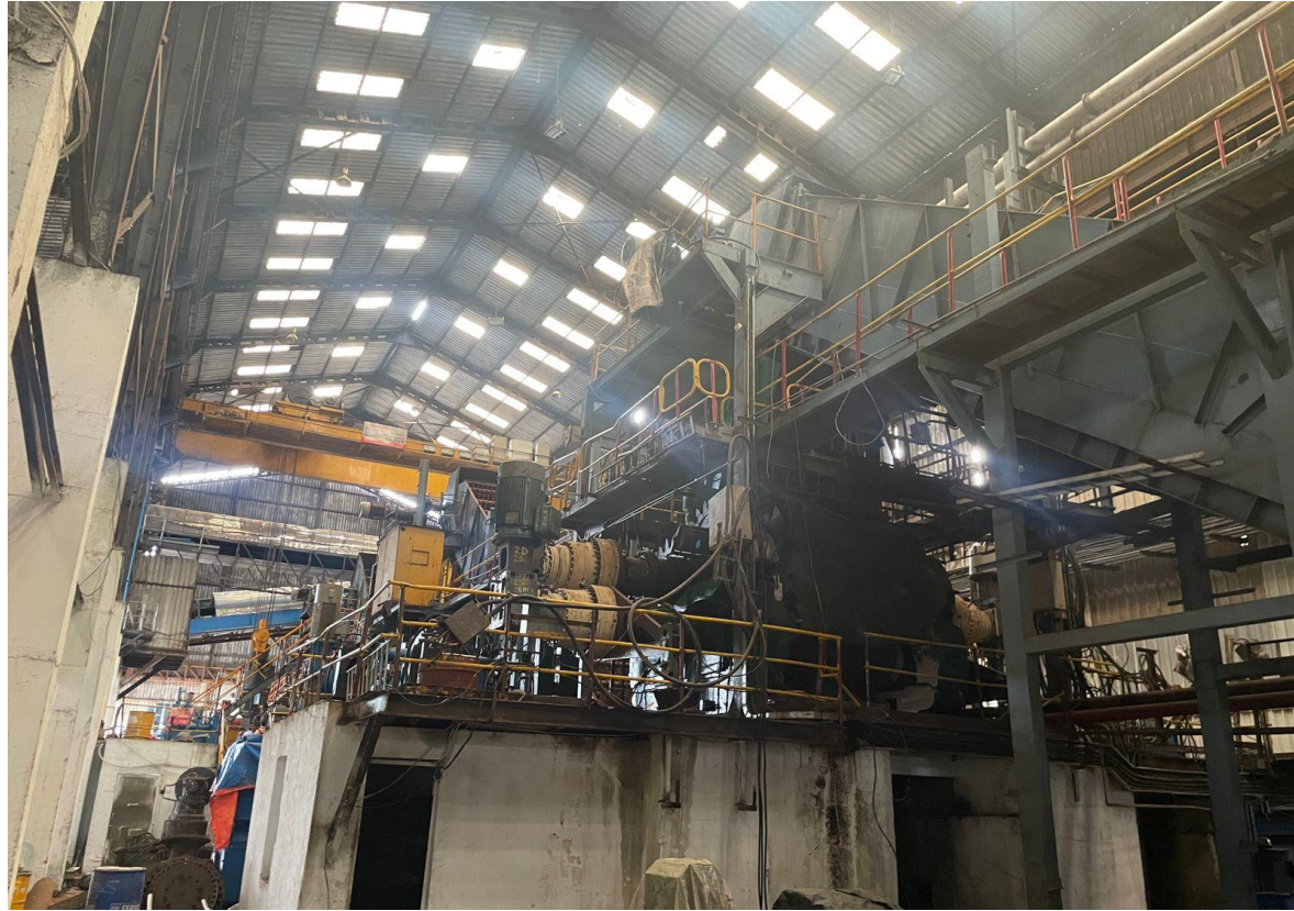
Picture 2: Mill house where the cane is crushed to extract juice and (b) Boiling house where impurities are removed from sugarcane juice
